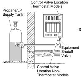
Figure 17 - Checking Gas Joints
